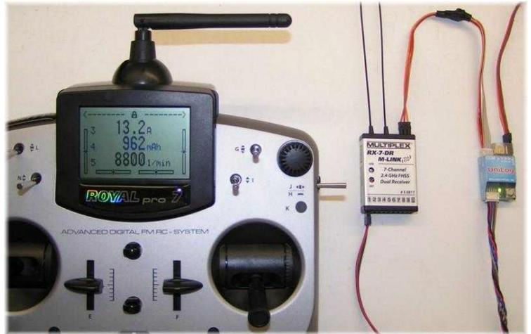
On the ground the data is displayed directly on the Multiplex Royal Pro or COCKPIT SX transmitters.
