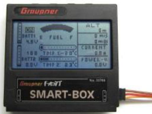
There are telemetry alarms for a maximum current, a minimum starting voltage, a minimum voltage, the maximum capacity and the maximum height. With the minimum starting voltage an uncharged battery accidentally connected can be detected, the maximum capacity allows flying to the desired value without inaccurate and cumbersome timers. The alarms are acoustically issued by the SMART-BOX and also shown in the display.
